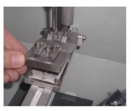
Easy replacement of nozzles. 4mm and 1.5mm can be changed to work as a standard air blasting cabin or as air jet erosion tester.
